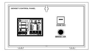
Datakom DKG307 digital automatic control module Hourmeter
