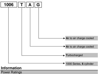
**Standby power rating** is for the supply of emergency power at variable load for the duration of the non-avalaibality of the mains power supply.No overload capacity is available at this rating.A standby rated engine should be sized for an avarage load factor of 80% based on published standby rating for 500 operating hours per year.Standby ratings should never be applied except
